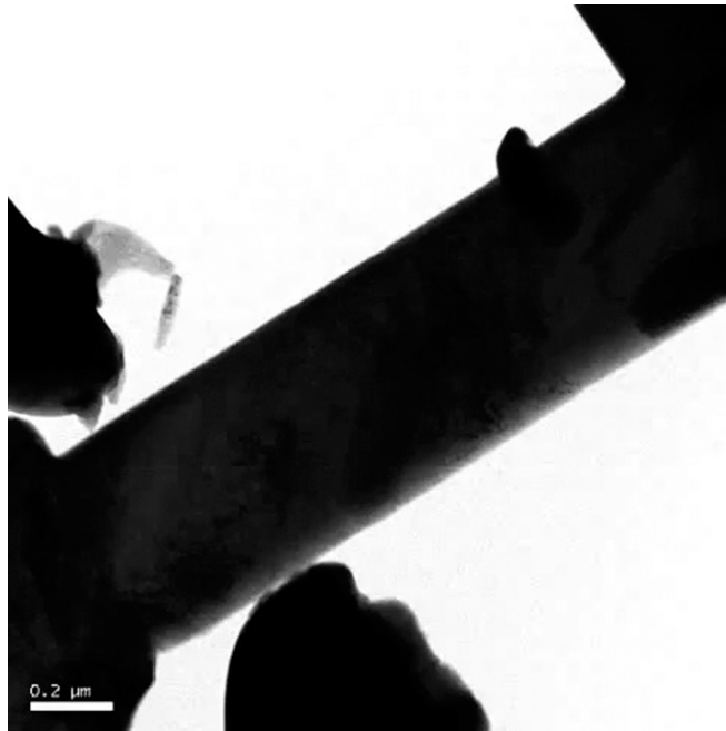
Movie S2. In situ TEM tensile test of a sample with a 600-nm gauge section.
