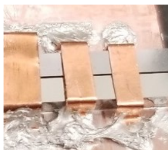
57 Fig. S3. Thermoelectric bars prepared for ion irradiation. Photograph of the two polished half-Heusler bars 58 prepared for irradiation with copper bridges suspended above selected regions of the bars.
